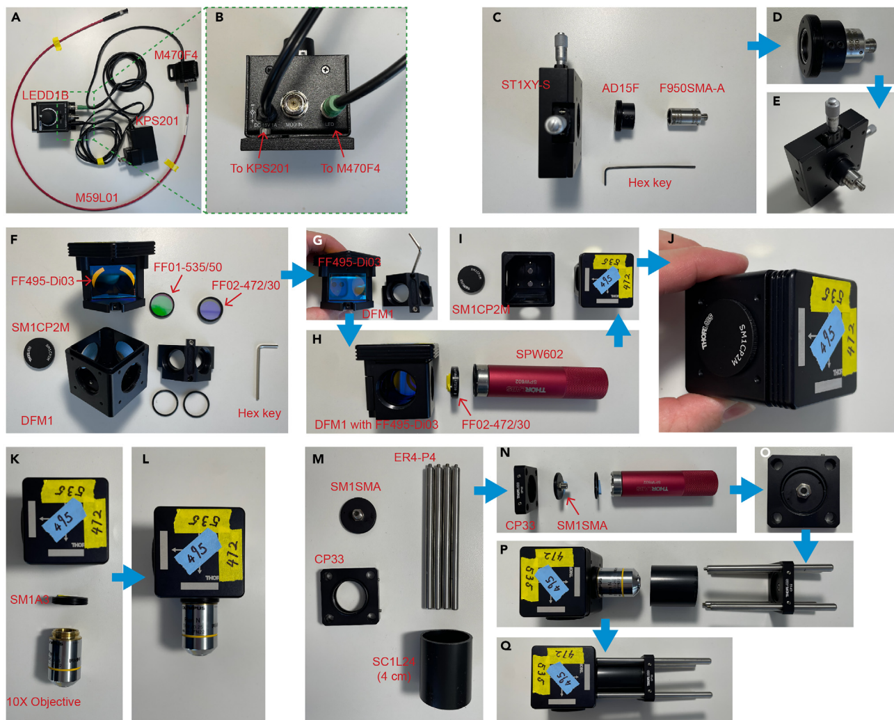
Figure 3. Step-by-step assembly of the multi-fiber photometry recording system (part I)
